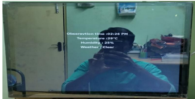
Figure 10: Weather status displayed in smart mirror
