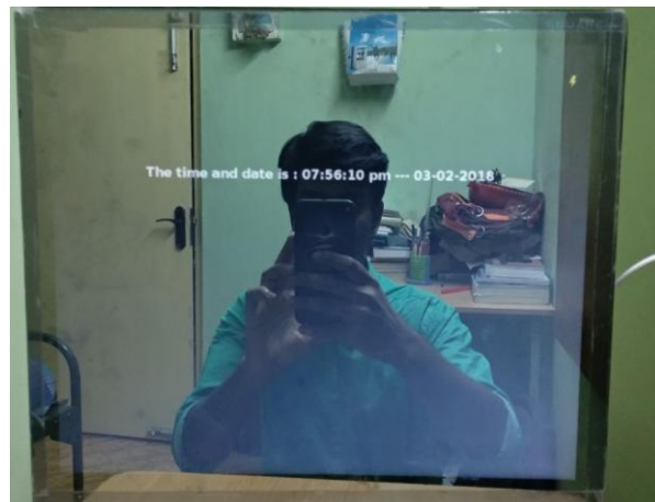
Figure 8: Time and date displayed in smart mirror
