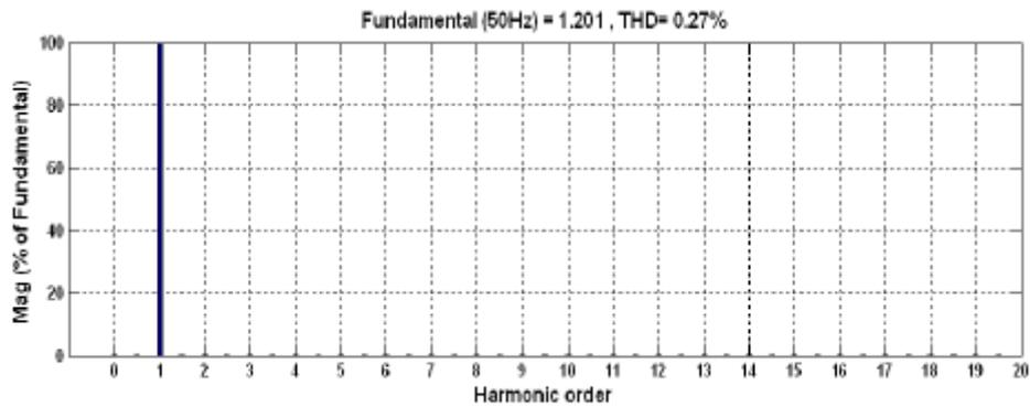
Fig. 7. Current waveform THD for five levels of output voltage of Fig.6.
