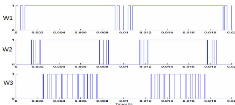
Fig. 4. Decision signals produced by the comparators.
