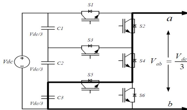
Fig. 2.2.2 Switching configuration required to produce output voltage level II.
