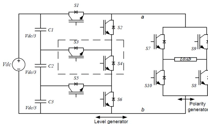
Fig. 2.1 configuration of presented single phase seven-level inverter.
