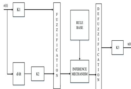
**Figure 3: basic structure of fuzzy logic controller**
