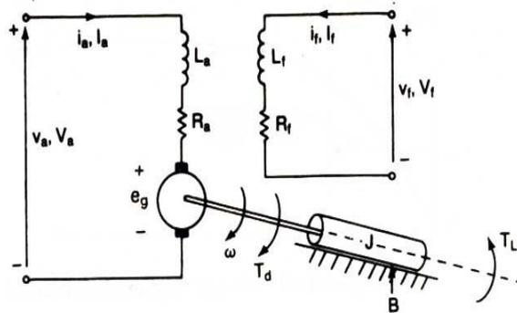
Figure 1: DC Motor Equivalent Circuit
