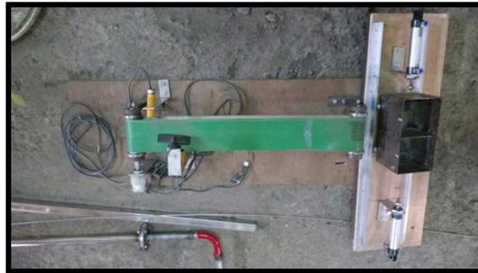
**Fig.3. Actual set up for the automated biscuit sorting**
