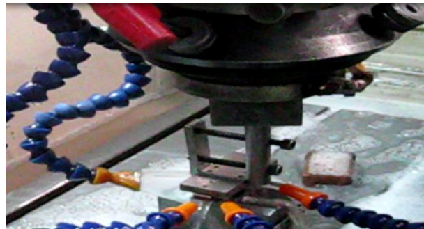
Fig.10 Parallality checking of electrode Fig. 11 Fabrication process of Microchannel Heat Sink
