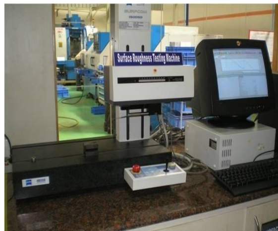
Fig.12 Equipment for Surface Roughness Measurement
