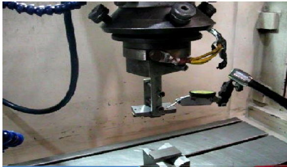
Fig.10 Parallality checking of electrode Fig. 11 Fabrication process of Microchannel Heat Sink
