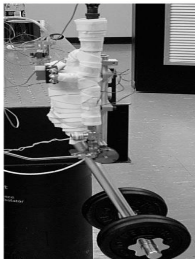
Fig. 6: Monopropellant actuator prototype wrapped with insulating tape and instrumented with thermocouples for measurement of surface temperature.
