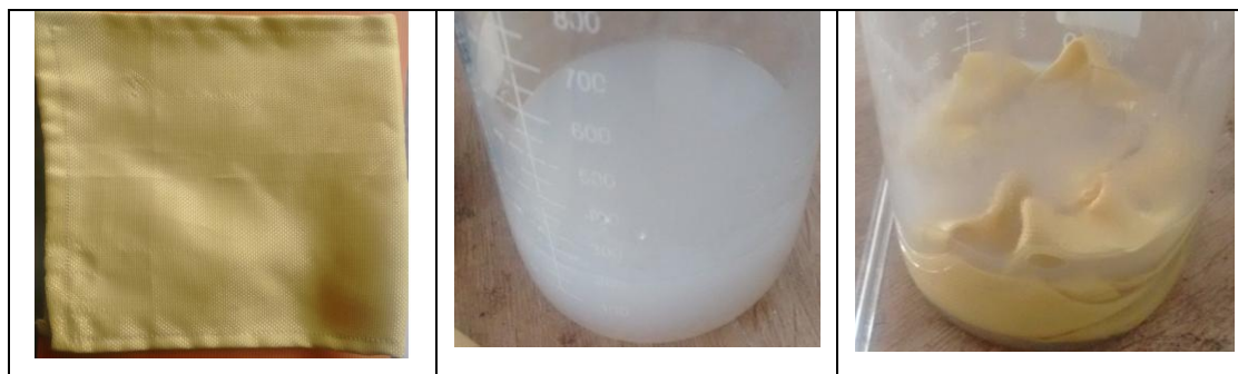
Figure (5):- The impregnation of nano particles solution can be done in two ways; By soaking, & by sandwiching the solution into layers.
