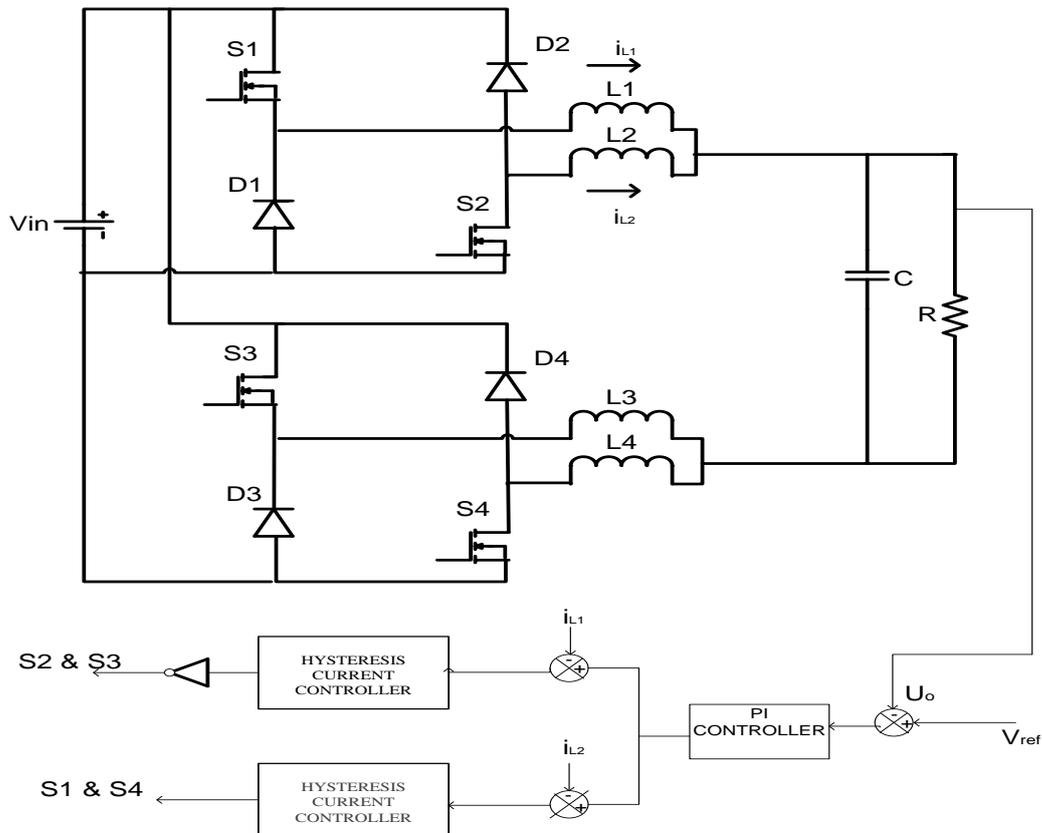
Fig. 1. DBFBI based Hysteresis current control
