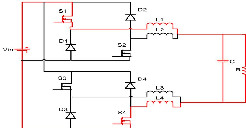
Fig. 2. DBFBI in Mode 1 for Positive Half Cycle
