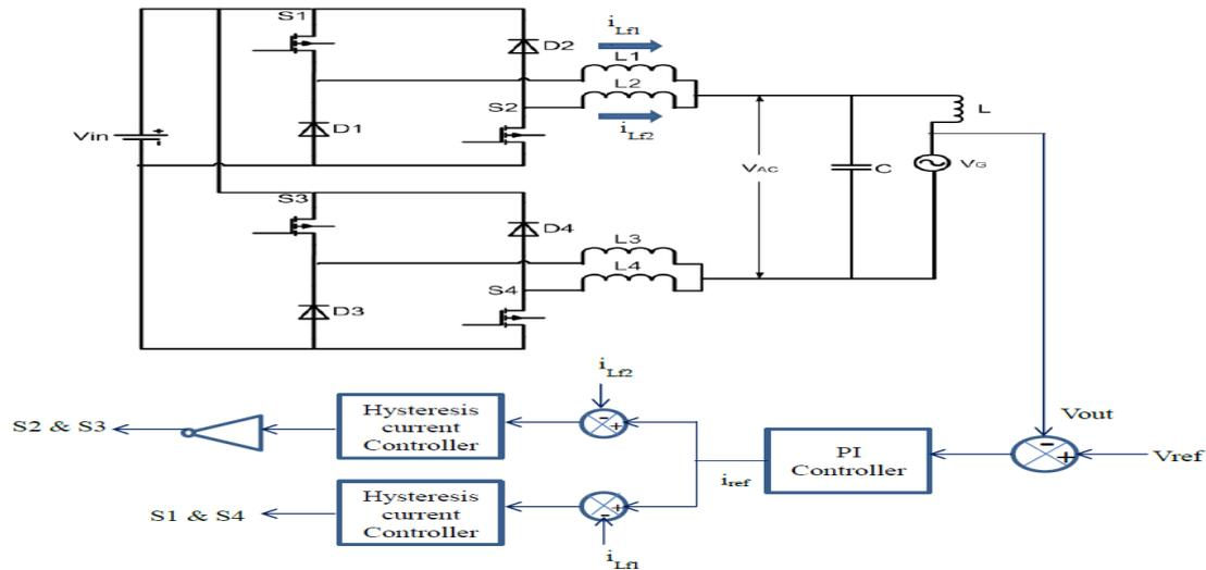
Fig.6 Complete Circuit and Block Diagram of Grid Connected DBFBI
