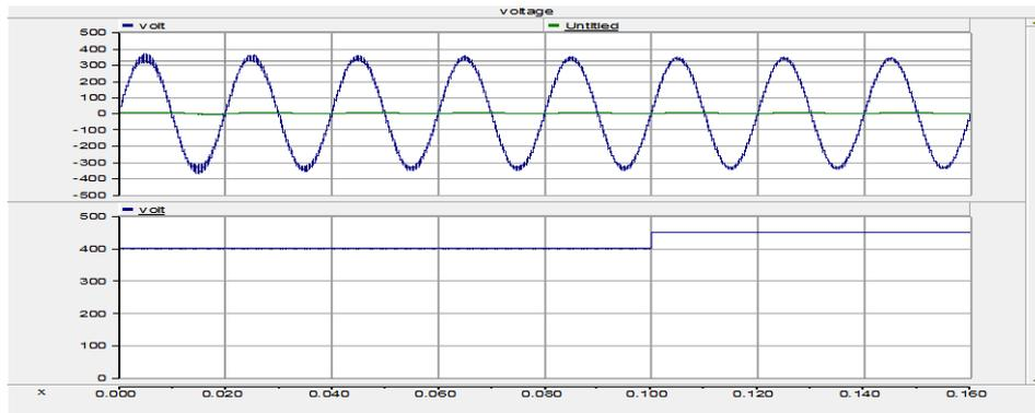
**Fig. 10. Input Voltage Disturbance and Corresponding Output Voltage**
