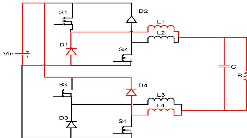
Fig. 3. DBFBI in Mode 2 for Positive Half Cycle
