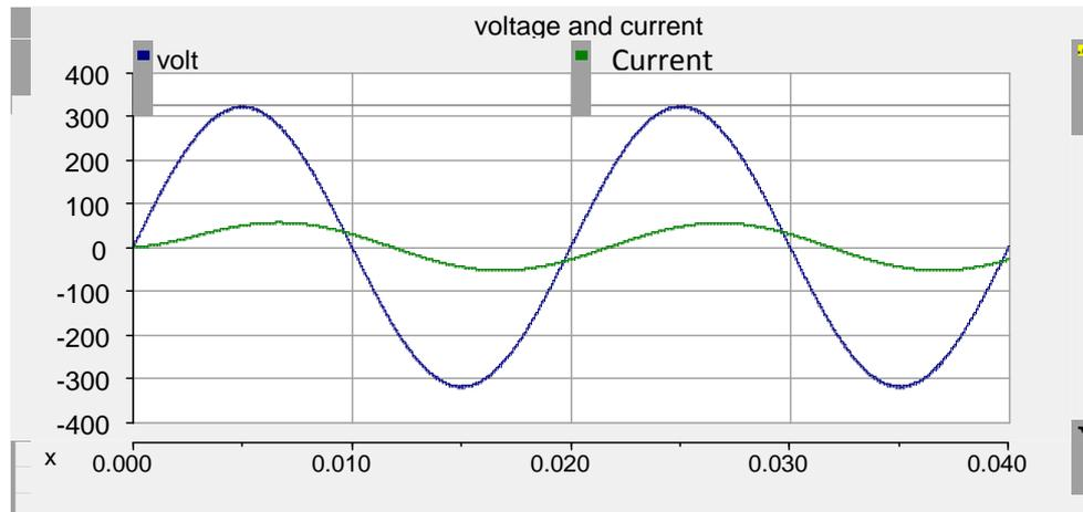
**Fig. 7. Closed Loop Output Voltage and Current Waveform (Current Scale Factor = 20)**
