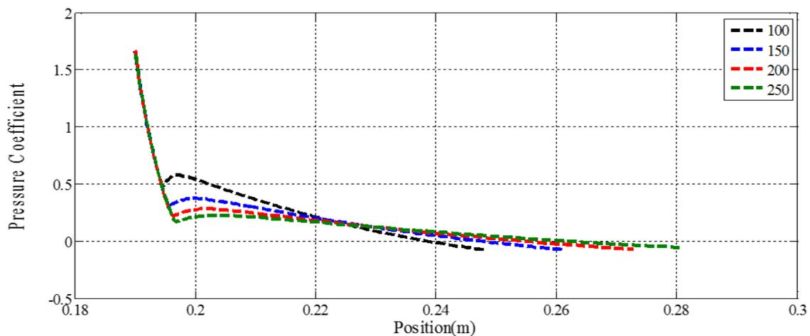
Fig. 4: Variation of pressure coefficient with upper body of a blunted tangent ogive at (a)  $r/R = 0.4$  ( $r = 10$  mm,  $R = 25$ mm) for (a)100mm (b)150mm (c)200mm (d)250mm
