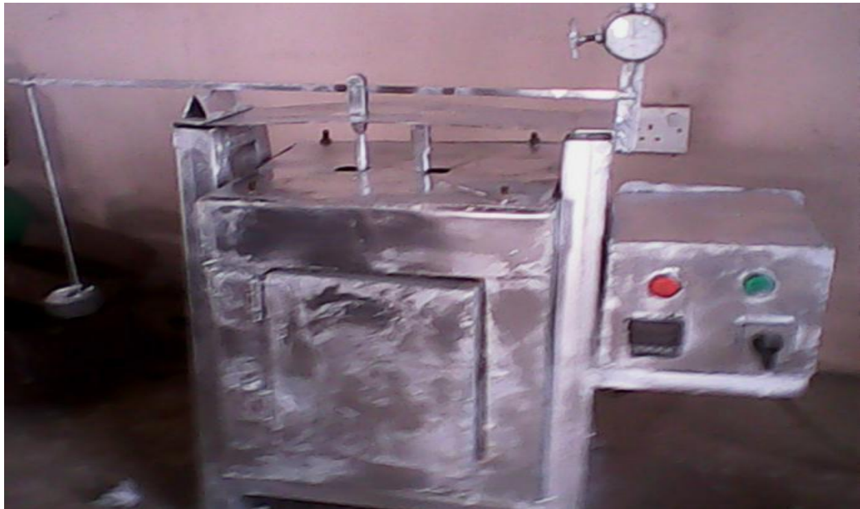
Figure.6: - (Complete Assembly Of Creep Testing Machine)
