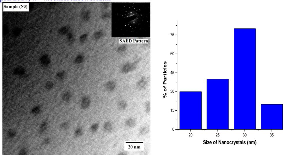
Figure 3.4: TEM image of sample N1, N2, N3 and histogram for annealed sample S3.
