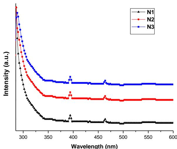
Figure 3.5: Absorption spectra of samples N1, N2 and N3.
