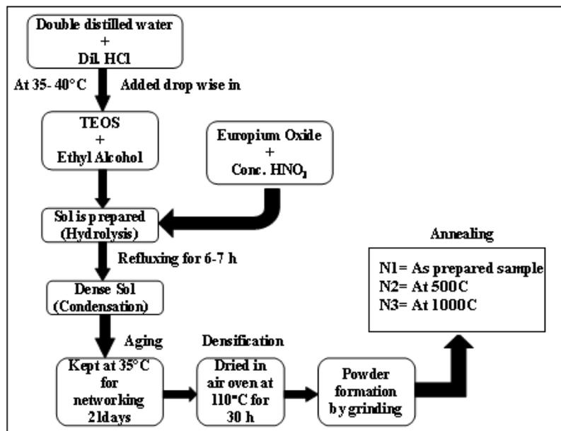
Figure 2.1: Block diagram of sample preparation using sol-gel process.
