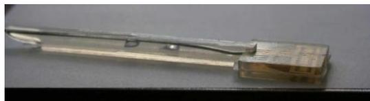
Fig. 4: Side view of antenna and cable embedded in PDMS[11]
