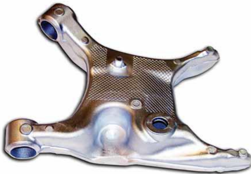
Figure 2 This rear lower control arm for the automotive industry was cast hollow with A356 aluminum alloy through a low-pressure permanent mold casting process [7]
