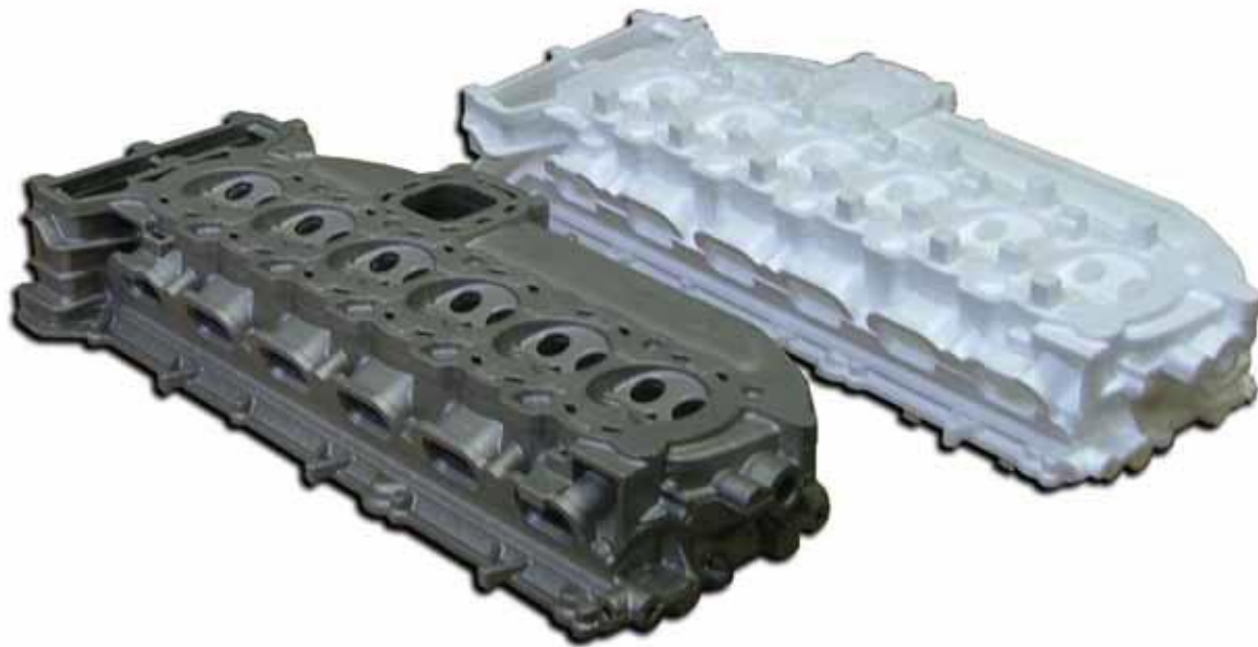
Figure 5 Cast with A356 aluminum alloy using the lost foam process, this verado L6 four-stroke cylinder head for a boat engine coupled an automotive-style cylinder head with a double-water jacketed exhaust manifold [7]
