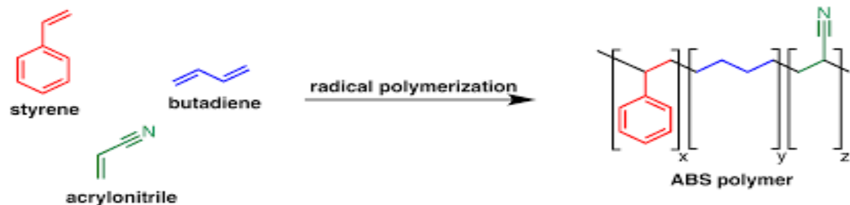
Fig. 1 monomer units and structure of ABS
