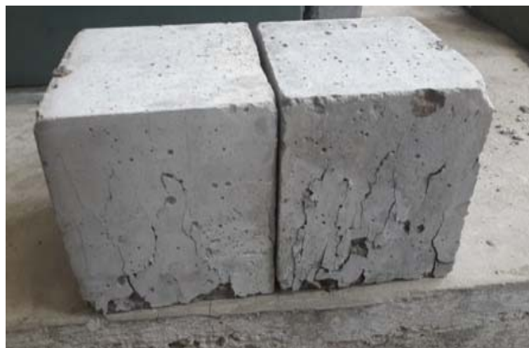
Fig -1: Crack Developed After Casting Of Cubes
