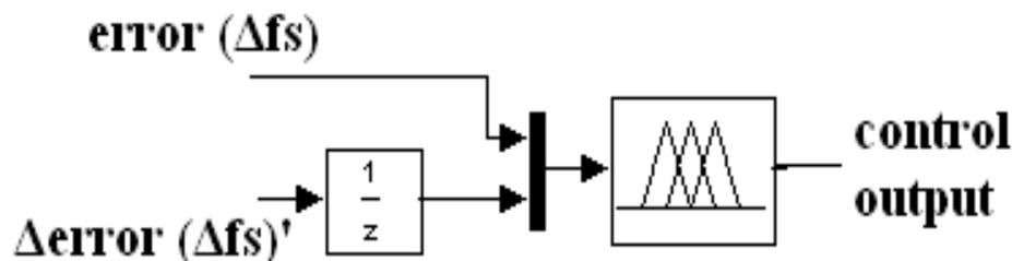
Fig 5: Block diagram of fuzzy logic controller
