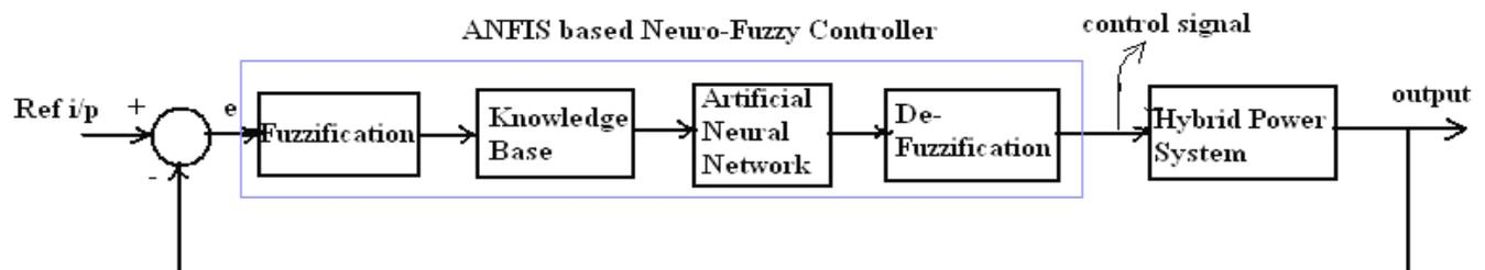
Fig 8: Block diagram of Neuro fuzzy controller
