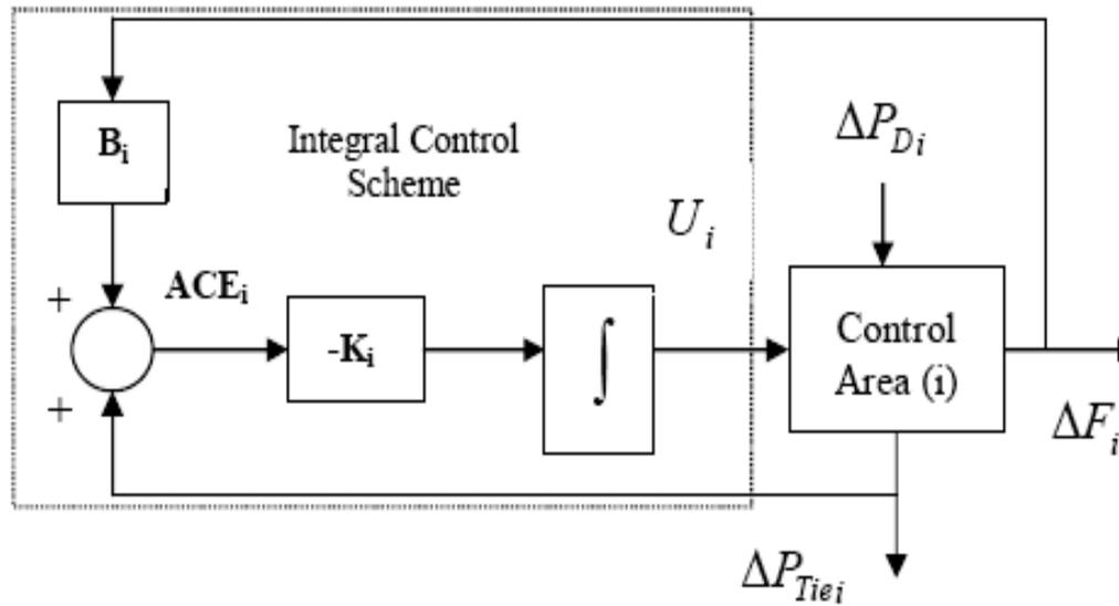
Fig 3: conventional PI controller connected in  $i^{th}$  area
