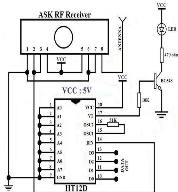
Figure 4: Receiver-Circuit Diagram
