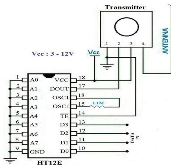
**Figure 3: Transmitter-Circuit Diagram**
