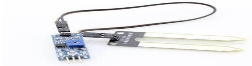
Probe is feedback instrument of the automated irrigation system. It used to measure moisture content of the soil. It is to be placed permanently. When it's getting activated, means of 5v supply then it sends electrical output signals which is given to the comparator circuit. This comparator circuit reads the signals, whose output is given to microcontroller.
