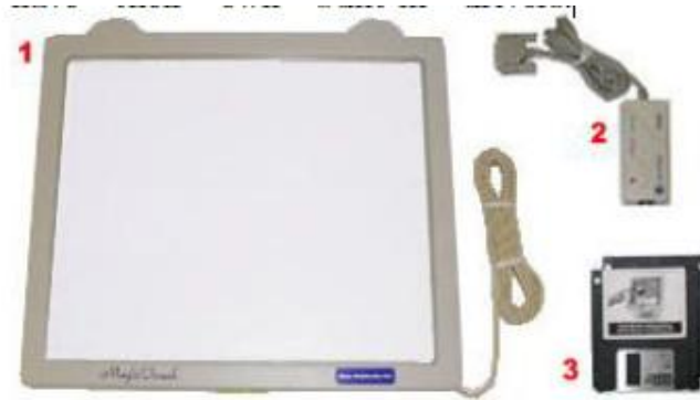
Fig. 6: components of touch screen [4].
