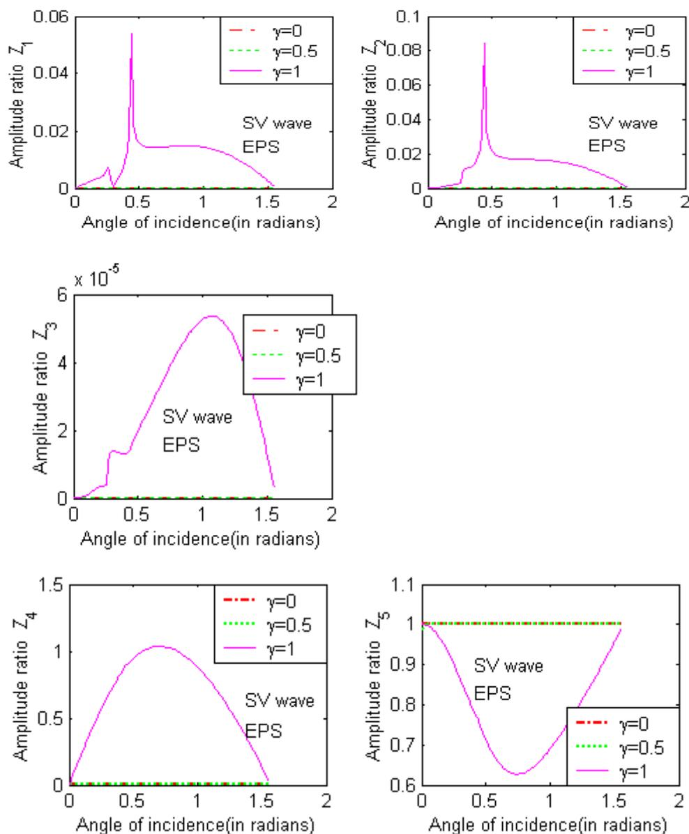
Figures 17-21. Variation of the amplitude ratios with angle of incidence of incident transverse wave showing porous effect
