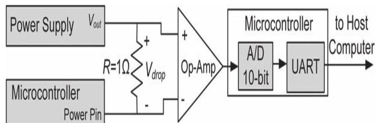
Fig. 3. Power measurement setup.
