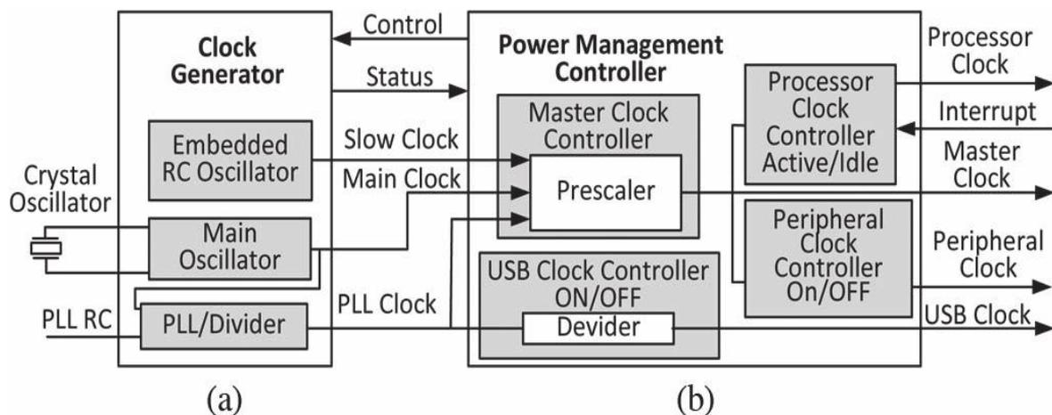
Fig. 2. Power management unit. (a) Clock generator. (b) Power management controller.
