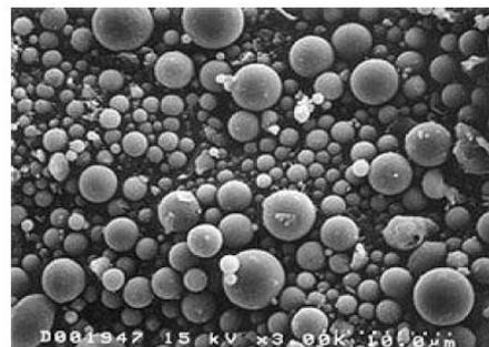
**Fig 3: SEM image of Fly ash**
