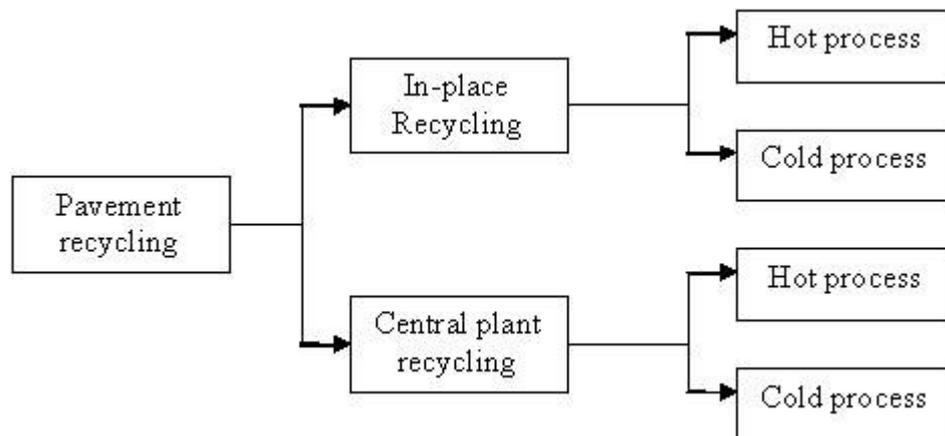
**Fig. Classification of recycling methods based on processes**
