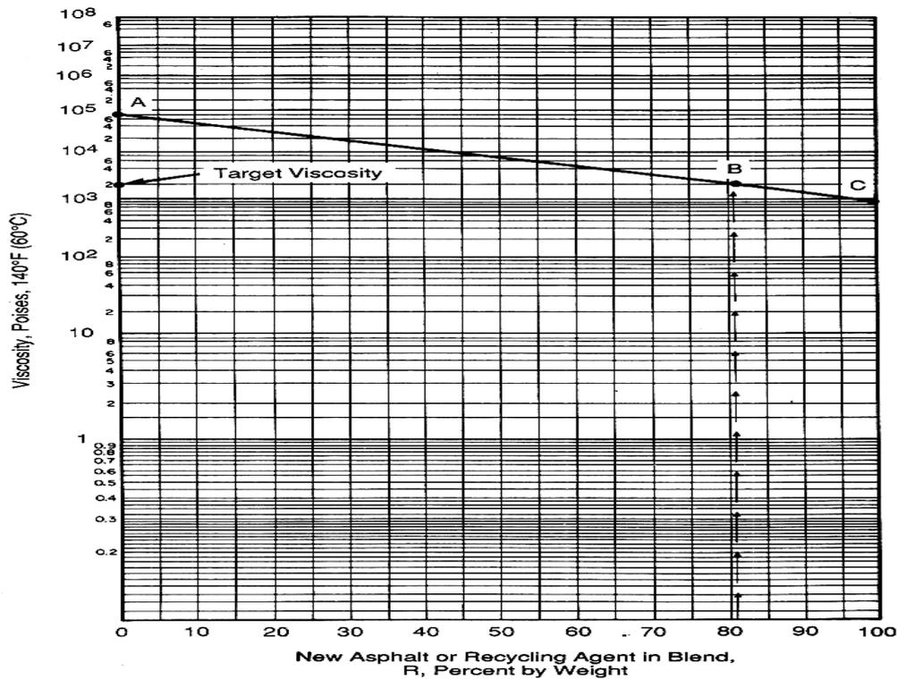
Figure A - Asphalt viscosity blending chart
