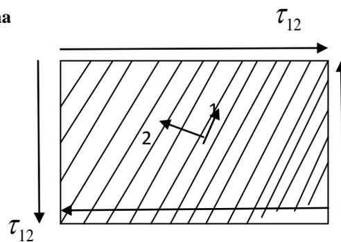
Fig. 4.4.2 Applied stresses in a unidirectional 20° lamina
