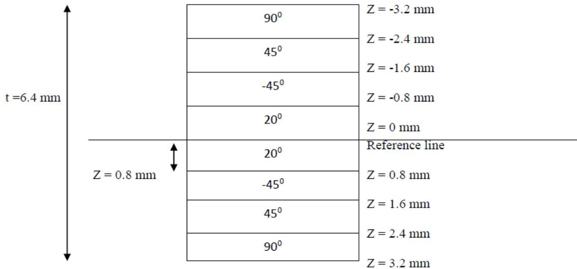
Fig 4.6 Thickness and coordinate location of the Eight-ply laminates [90/ 45/ -45/ 20],
