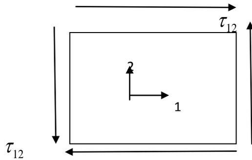
Fig. 4.4.1 Applied stresses in a unidirectional 0° lamina
