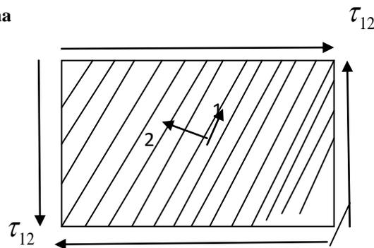
Fig. 4.4.3 Applied stresses in a unidirectional 45° lamina
