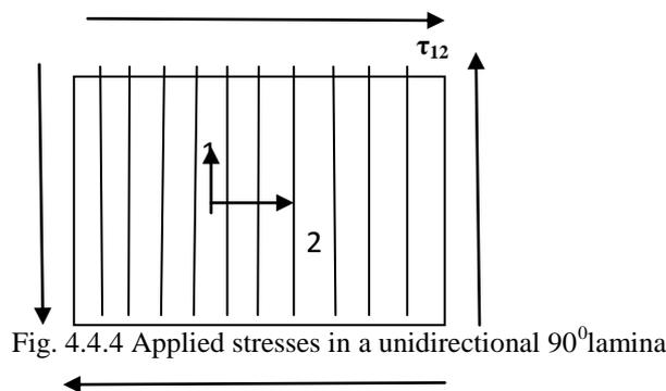
Fig. 4.4.4 Applied stresses in a unidirectional 90° lamina
