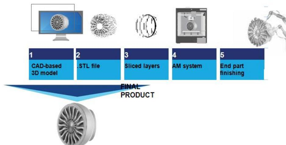
Figure 1. Additive manufacturing (AM) process flow
