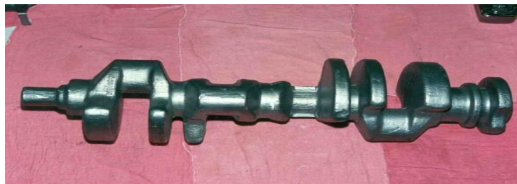
Fig. 3.1. Two-Plane V8 Crankshaft Raw Forging.
