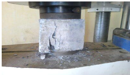
Fig.2 Compression strength test under UTM
