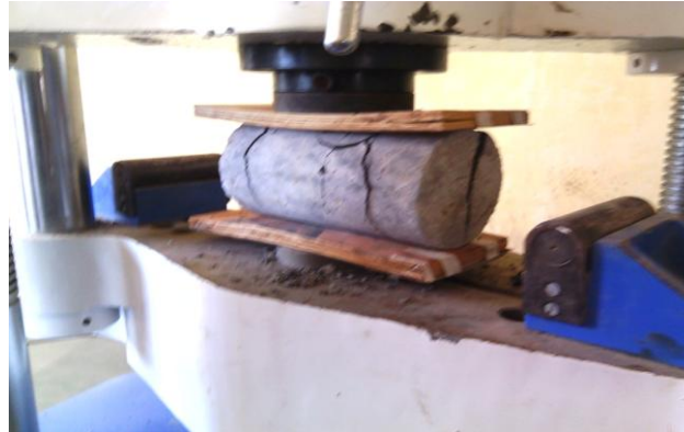
Fig. 3 Split Tensile strength test for cylinder
