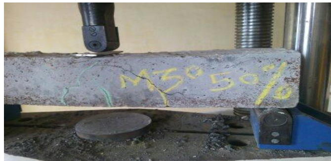
Fig.4 Flexural strength of beam.
