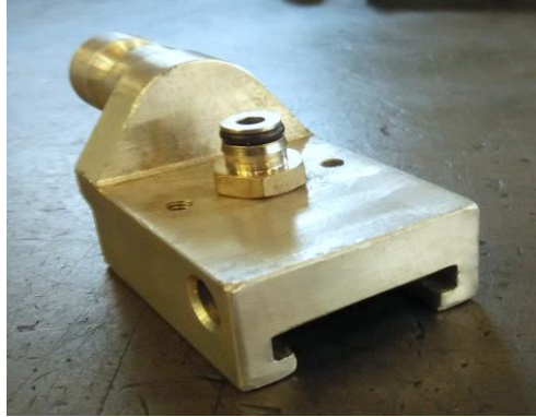
Fig.6.3.2 Manufactured suction pad attacher with mounting elements.
