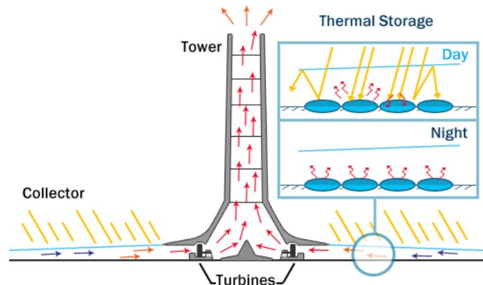
**Fig.1. Working principle of solar updraft tower [1].**
