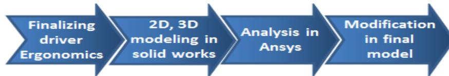
Fig.1 Design Methodology of Roll Cage
