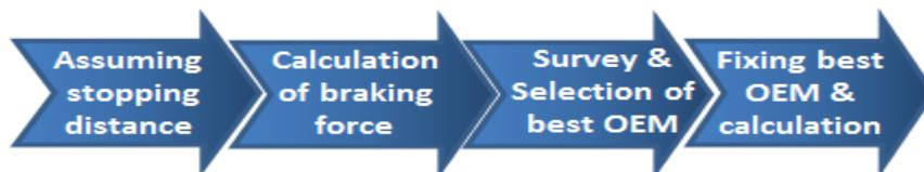
**Fig.8 Design methodology of braking system**
