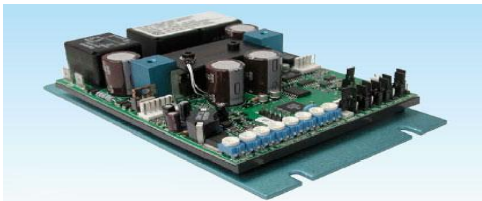
Figure 10: KBBC-24M controller for the steering actuator
