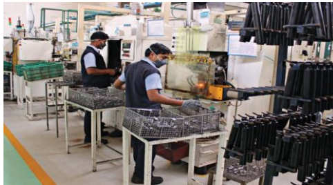
Welding line for Monoshocks
