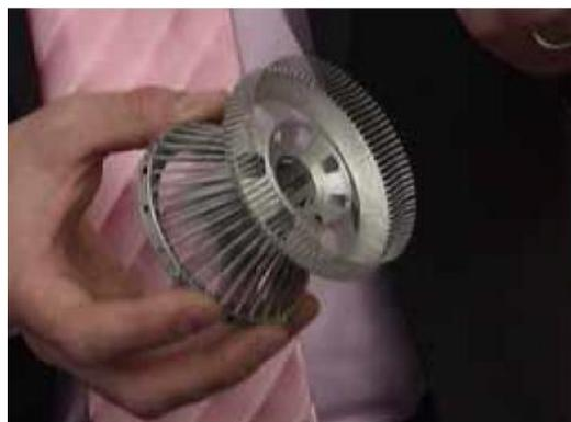
**Figure-4.2 A few engineering parts generated on METAL RPT**
