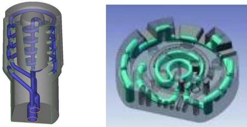
**Figure-4.3 An example of moulds with Conformal cooling channels**
