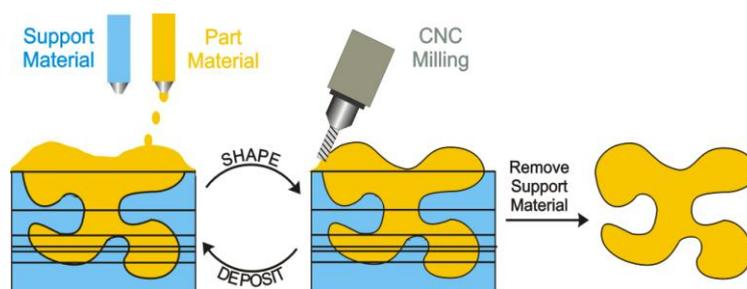
Figure 1 - Shape Deposition Manufacturing (Cross-sectional View)
