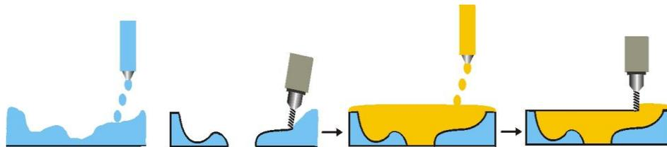
**Figure 3. Example of a deposition and shaping sequence**
