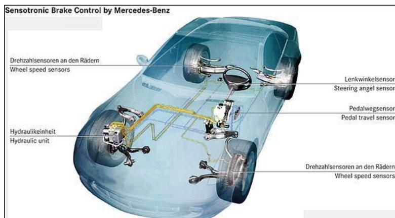
When drivers hit the brake pedal today, their foot moves a piston rod which is linked to the brake booster and the master brake cylinder. Depending on the pedal force, the master brake cylinder builds up the appropriate amount of pressure in the brake lines which - in a tried and tested interaction of mechanics and hydraulics - then presses the brake pads against the brake discs via the wheel cylinders.
