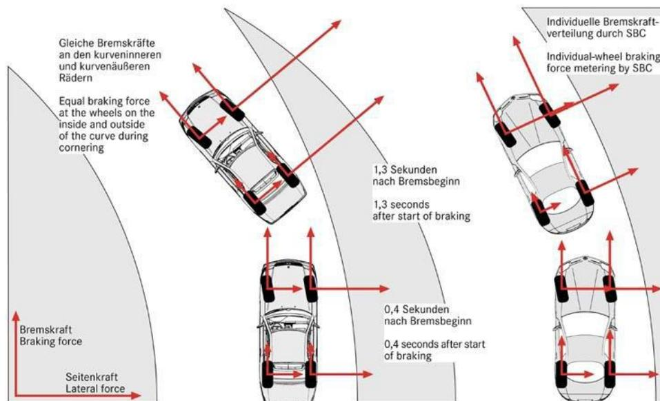
**Braking in a curve. Left: conventional. Right: with SBC.**
