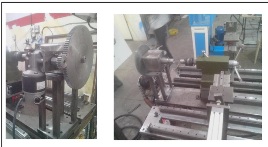
Fig.4.1 Assembly of Head Stock and Tail Stock
