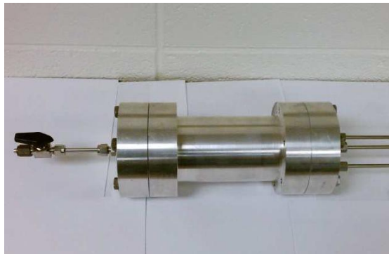
Fig.1.2 Metal hydride tank
