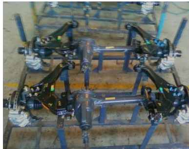
4 wheel drive axle assembly used for scorpio
