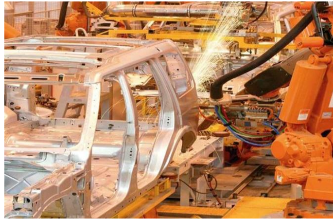
Fig. 2 Industrial robots welding car body (Source: Rexroth- Bosh group) [4]
