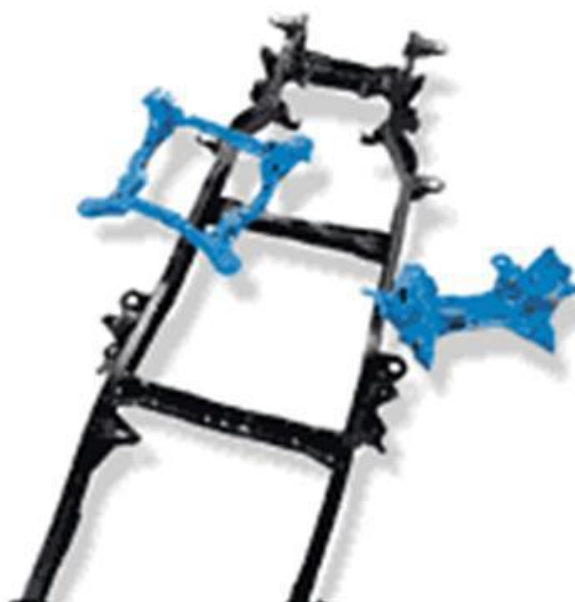
Fig. 10 Automobile components (frames) produced by MPW process
