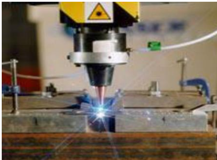
Fig. 8 Laser beam welding of low carbon steel sheet
