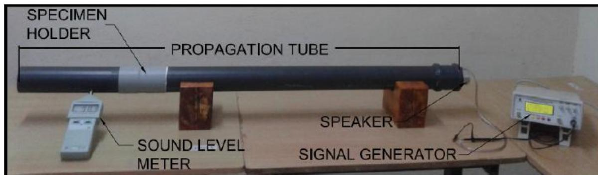
**Fig.2 Impedance Tube System for Sound absorption Measurement**
