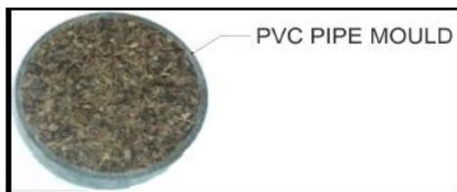
**Fig.1 Mould used for Specimen Casting**
