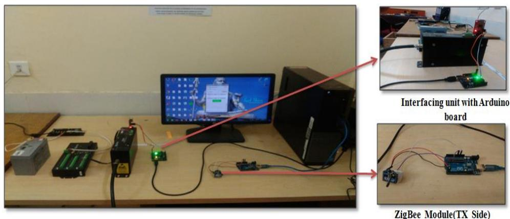
**Fig.3 The lab set up including transmitter side**
