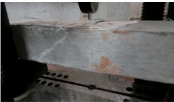
Fig. 9: Failed beam BS6 after testing
