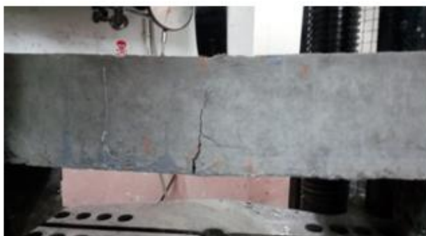
Fig. 13: Failed beam BF4 after testing
