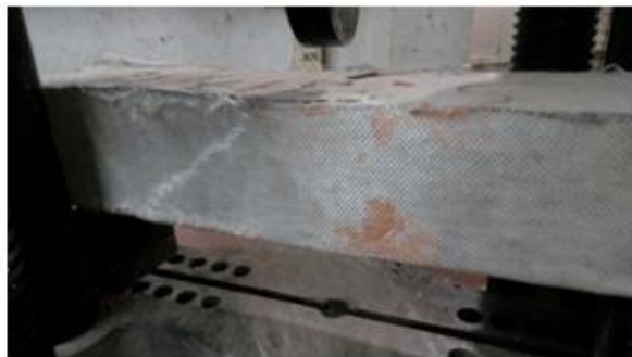
Fig. 3: Failed beam S1 after testing
