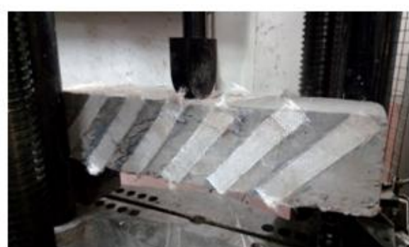
Fig. 6: Failed beam BS3 after testing
