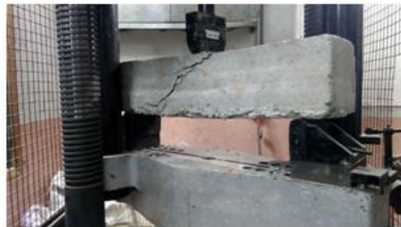
Fig. 4: Failed beam CBS1 after testing
