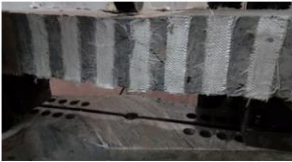
Fig. 7: Failed beam BS4 after testing
