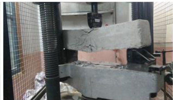
Fig. 12: Failed beam BF3 after testing
