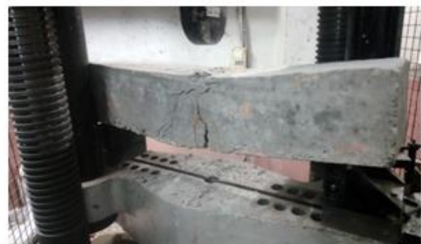
Fig. 10: Failed beam CBF1 after testing
