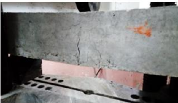
Fig. 11: Failed beam BF2 after testing
