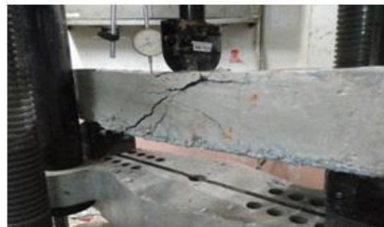
Fig. 2: Failed beam F1 after testing
