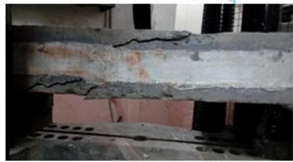
Fig. 8: Failed beam BS5 after testing
