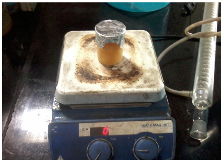
Fig 6 Preparation of nanofluid using magnetic stirrer
