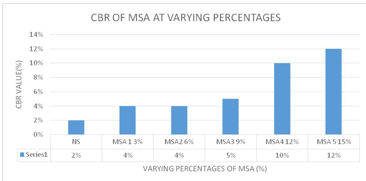
**Fig.7. CBR values of MSA mixed with soil.**
