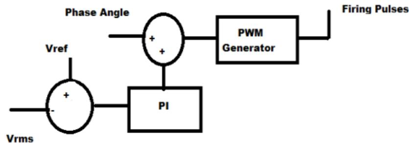
Fig 5. Block Diagram of PI Controller
