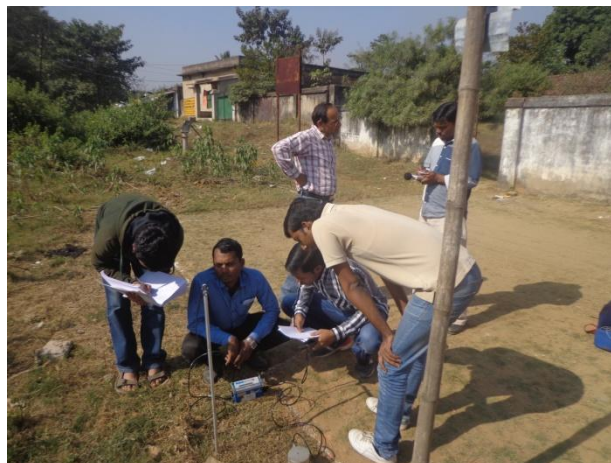
Fig.3. monitoring of ground vibration with minimate
