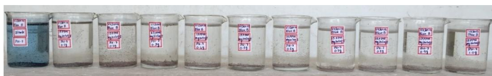
Photo 1: Effect of catalyst concentration on VBB at 120 minutes [VBB=15 ppm, pH=7, MgZnSrO 3 (urea)]
