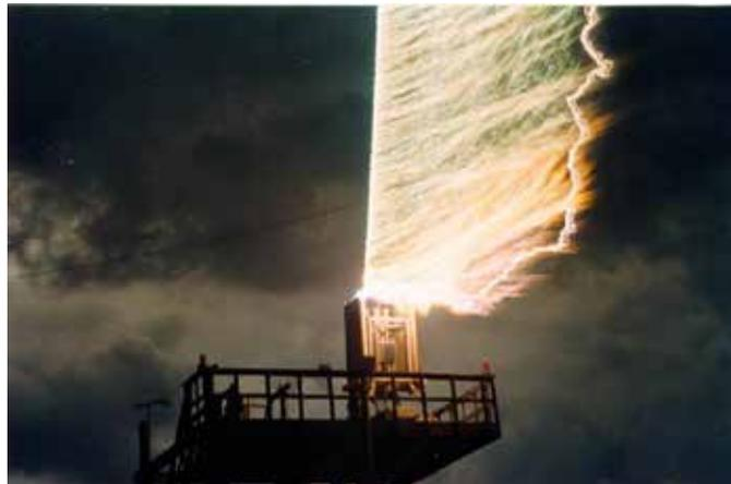
**Fig. 6 Invoking and carrying of lightning using a conductor**
