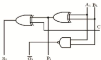
FIG: 4 Modified Full Adder
